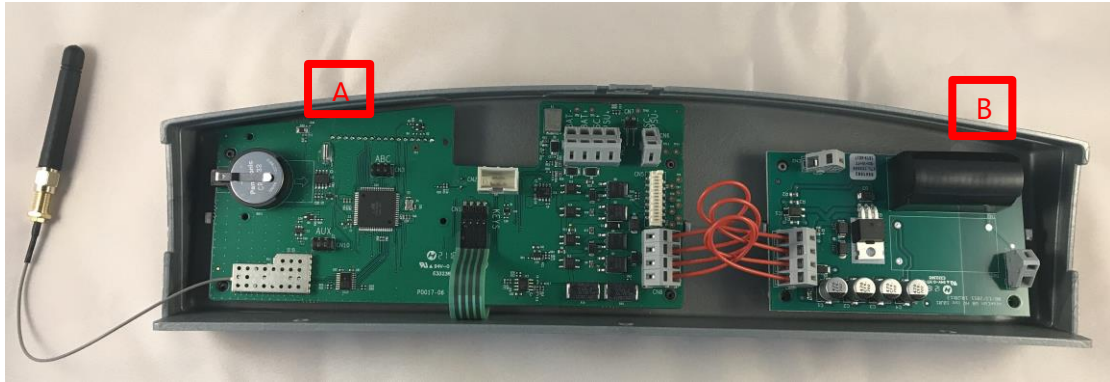
Figure 5: Inside of control panel. A) Is the control PCB. B) Is the separated high voltage generating PCB.
