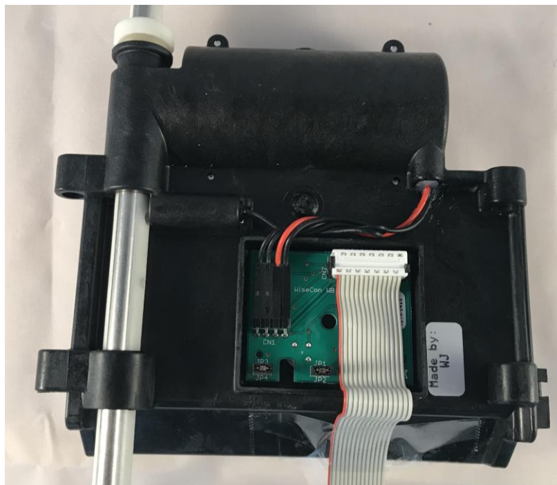
Figure 17: Elevator seen from the back before elevator PCB is enclosed in Iso-pur k 760 epoxy.
