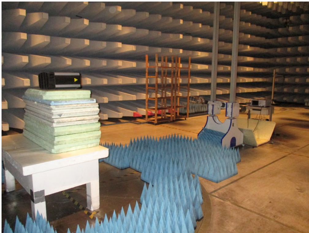
Photo 2.8 Test set up regarding measurement of radio frequency electromagnetic field above 1 GHz. Horizontal orientation
