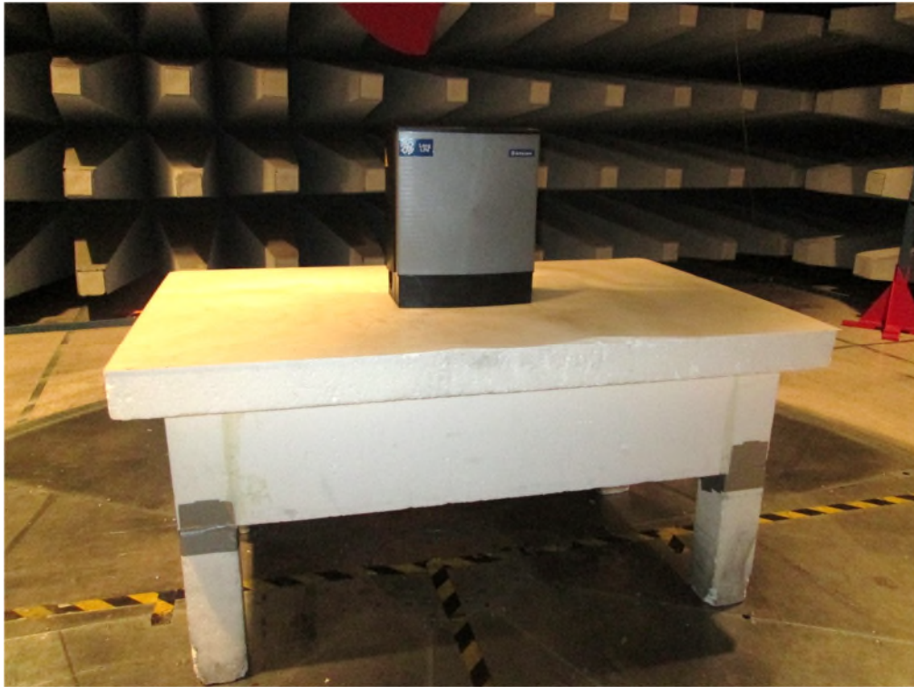
Photo 2.1 Test set up regarding measurement of radio frequency electromagnetic field below 1 GHz.
