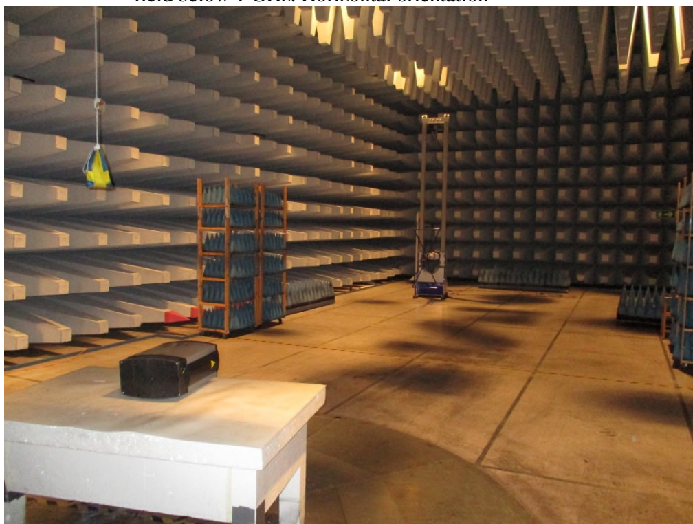
Photo 2.4 Test set up regarding measurement of radio frequency electromagnetic field below 1 GHz. Horizontal orientation
