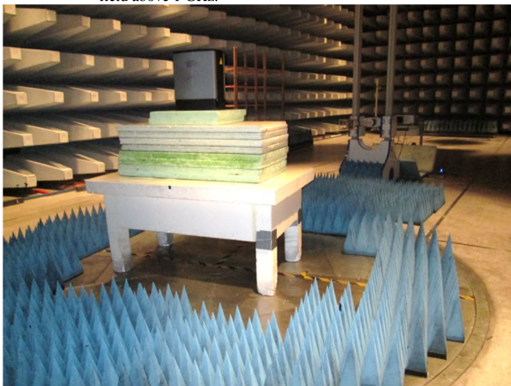
Photo 2.6 Test set up regarding measurement of radio frequency electromagnetic field above 1 GHz
