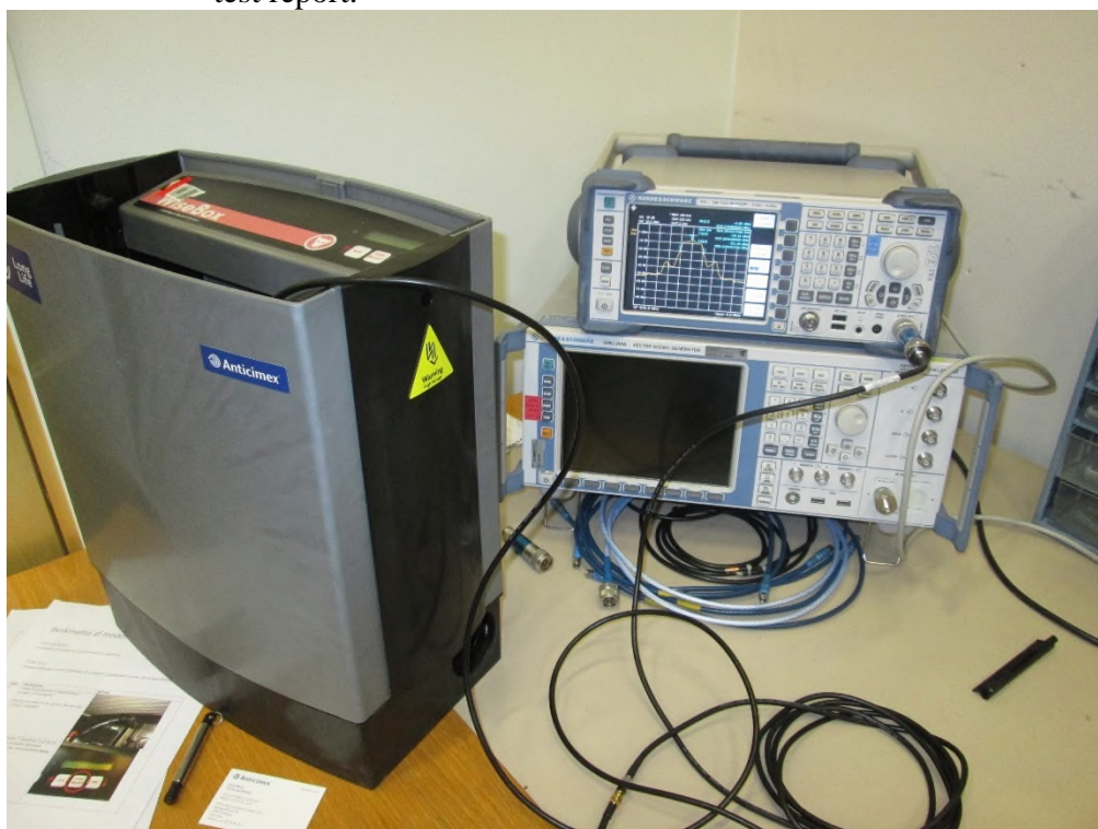
Photo 2.10 Test set up regarding radio parameter tests in chapter 4.3, 4.6 and 4.7 in test report.
