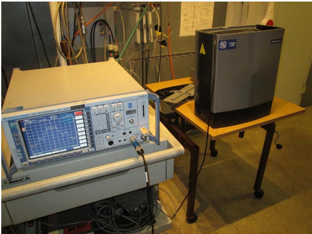
Photo 4.4.2 Test setup regarding measurement of 6 dB bandwidth.
