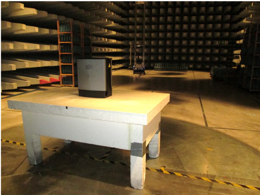
Photo 4.1.2 Test setup regarding measurement of radio frequency electromagnetic field.
