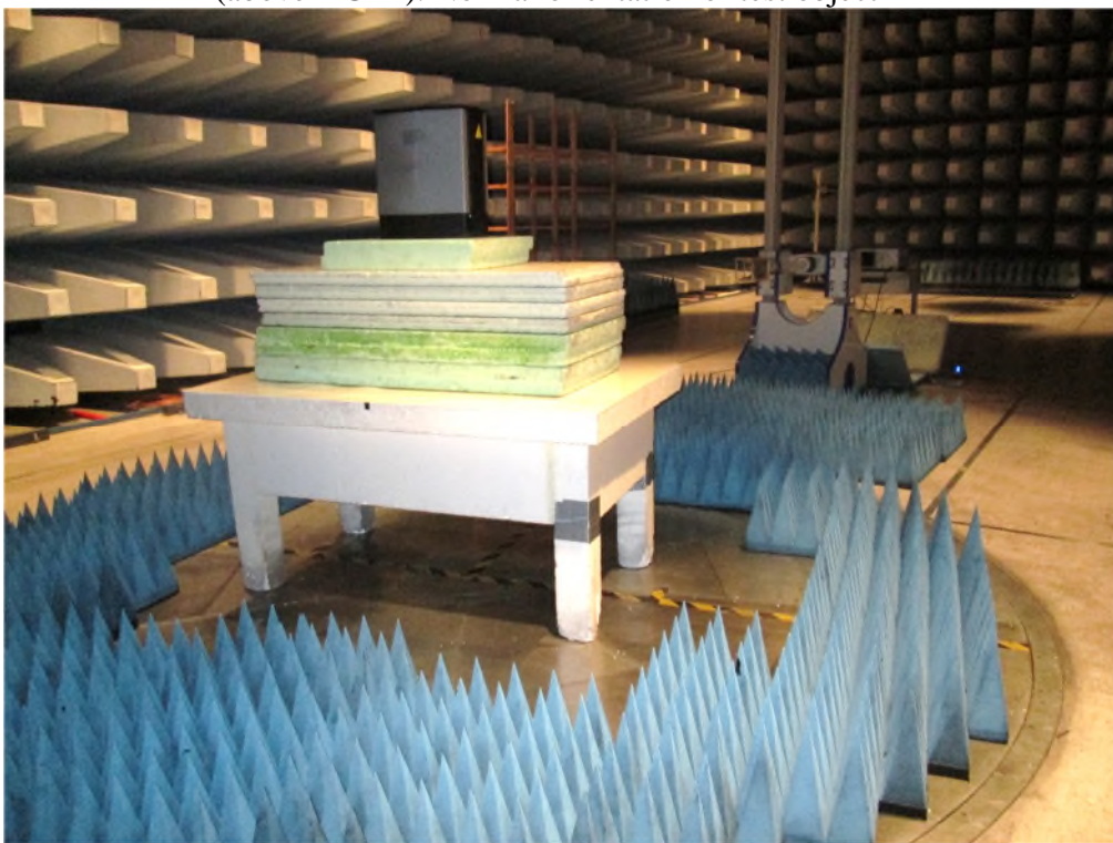
Photo 4.2.2 Test setup regarding measurement of radio frequency electromagnetic field (above 1 GHz). Normal orientation of test object
