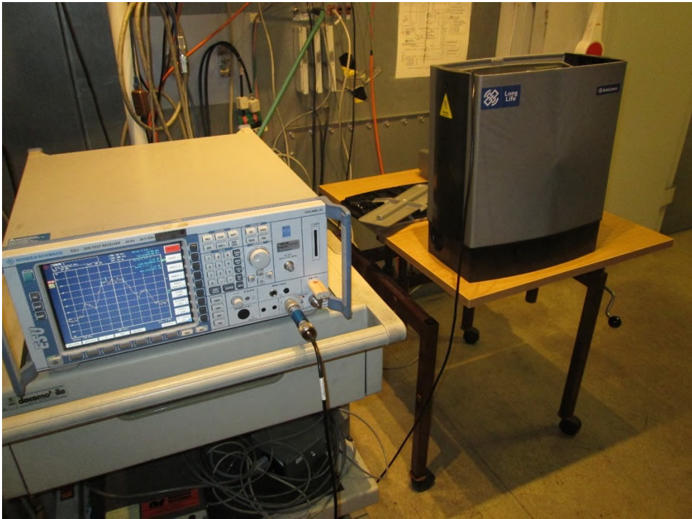
Photo 4.5.2 Test setup regarding measurement of 20 dB bandwidth.
