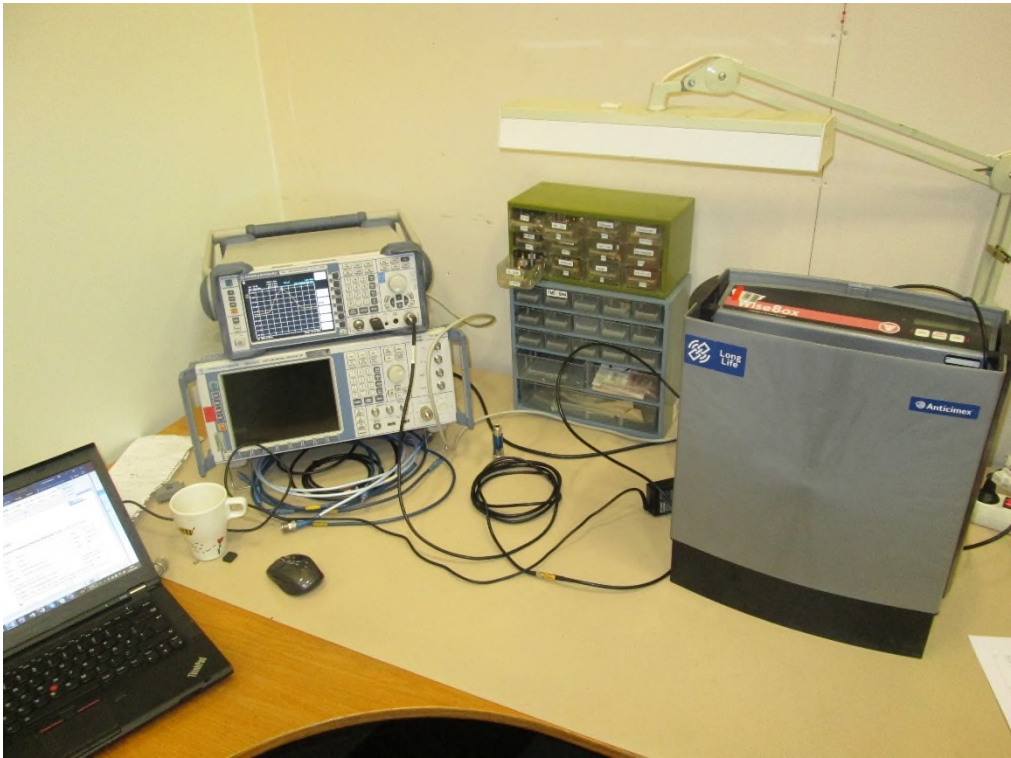
Photo 4.3.2 Test setup regarding measurement of maximum conducted output power.
