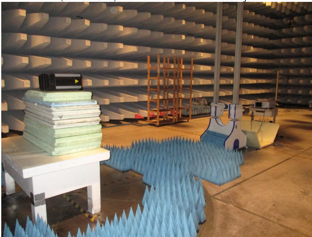
Photo 4.2.4 Test setup regarding measurement of radio frequency electromagnetic field (above 1 GHz). Horizontal orientation of test object
