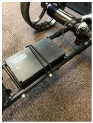
Next, strap the battery down on the cart so it does not move during operation.
