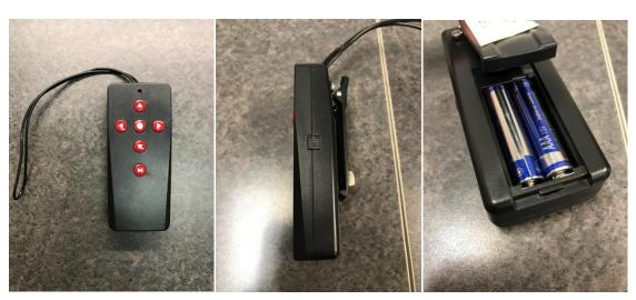
To turn the remote on, slide the switch on the side of the remote towards the antenna. The cart has three speeds in each direction:
