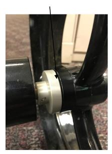
The rear wheelie bar will also need to be attached for use. In order to attach, pull up on the knob located on the wheel and slide the wheelie bar onto the square bar on the back of the cart. The Wheelie bar will lock into the corresponding hole on the cart. The wheelie bar will "click" into place.
