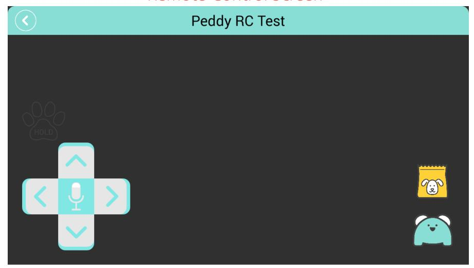
Once you press the HOLD button to activate direction keys (front, rear, left, right), you can make Peddy keep moving without pressing the HOLD button. If you press the STOP button or SNACK button, the function temporarily stops.
