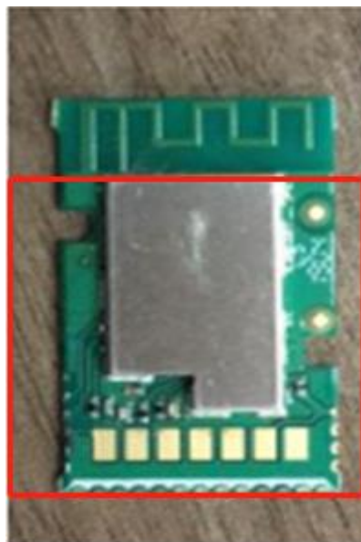
Drawing 2-3 Description of Clear Area of Antenna
