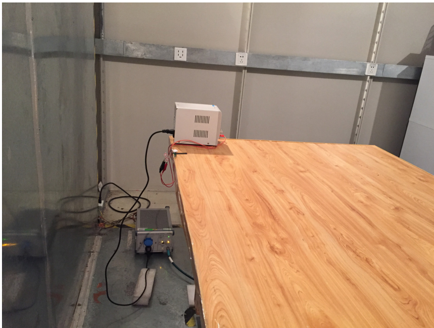
Conducted Emissions (Side View)
