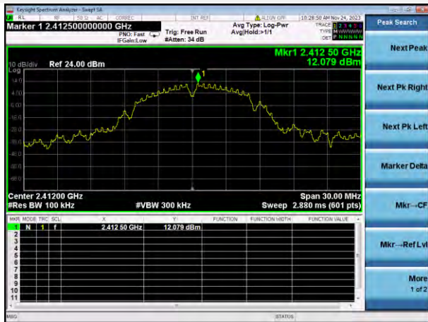
802.11b LOW CHANNEL, CARRIER LEVEL
