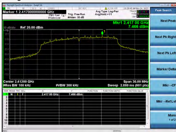
802.11g LOW CHANNEL, CARRIER LEVEL
