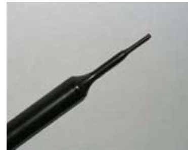
Picture C.2 Near-field Probe
