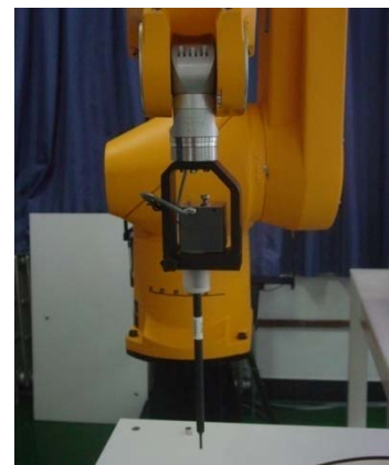
Picture C.3 E-field Probe
