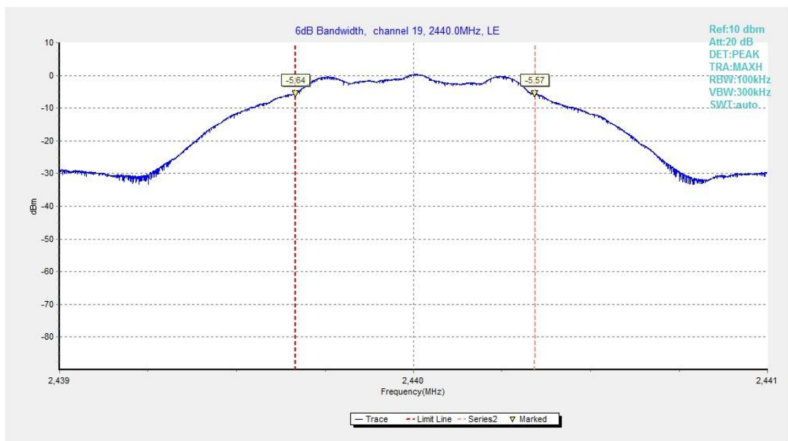
Fig.21. 6dB Bandwidth: GFSK, 2440 MHz
