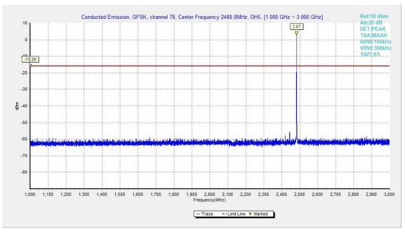
Fig.25. Conducted spurious emission: GFSK, Channel 78, 1GHz - 3GHz
