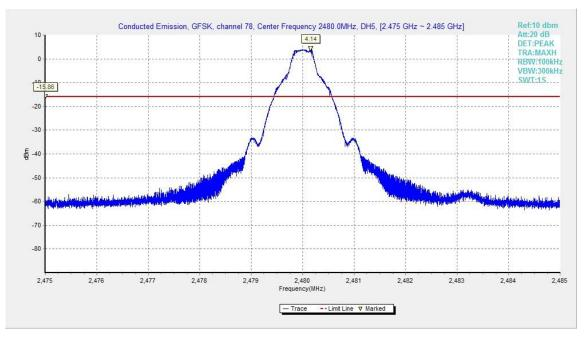
Fig.23. Conducted spurious emission: GFSK, Channel 78, 2480MHz
