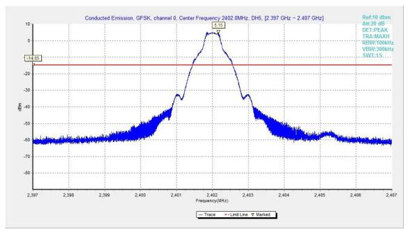
Fig.13. Conducted spurious emission: GFSK, Channel 0,2402MHz
