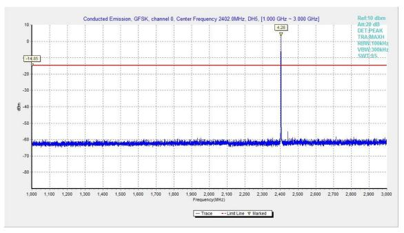
Fig.15. Conducted spurious emission: GFSK, Channel 0, 1GHz - 3GHz
