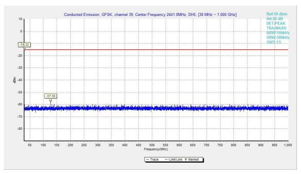
Fig.19. Conducted spurious emission: GFSK, Channel 39, 30MHz - 1GHz
