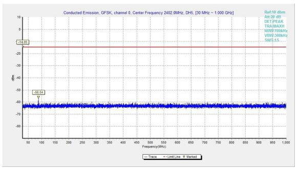
Fig.14. Conducted spurious emission: GFSK, Channel 0, 30MHz - 1GHz
