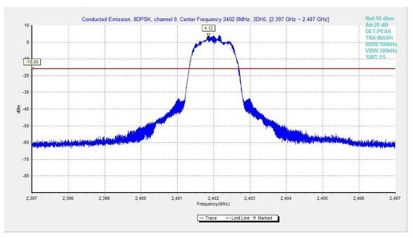
Fig.43. Conducted spurious emission: 8DPSK, Channel 0,2402MHz
