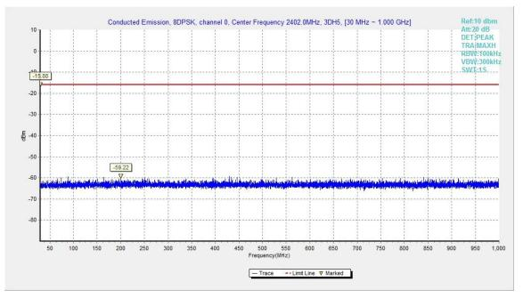
Fig.44. Conducted spurious emission: 8DPSK, Channel 0, 30MHz - 1GHz
