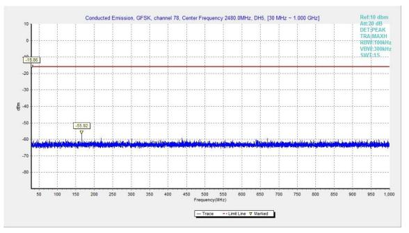
Fig.24. Conducted spurious emission: GFSK, Channel 78, 30MHz - 1GHz
