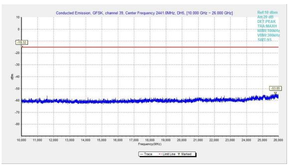
Fig.22. Conducted spurious emission: GFSK, Channel 39, 10GHz - 26GHz
