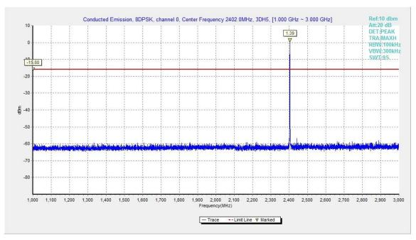
Fig.45. Conducted spurious emission: 8DPSK, Channel 0, 1GHz - 3GHz
