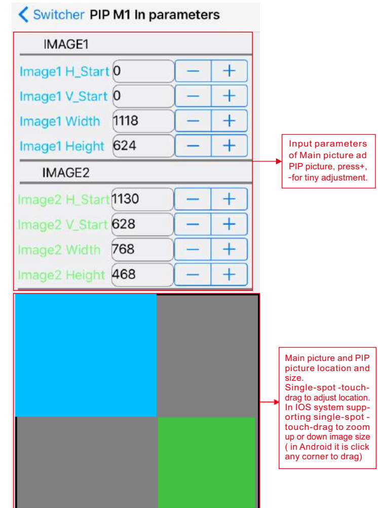
Pic 8-3j PIP input / output parameters setting interface
