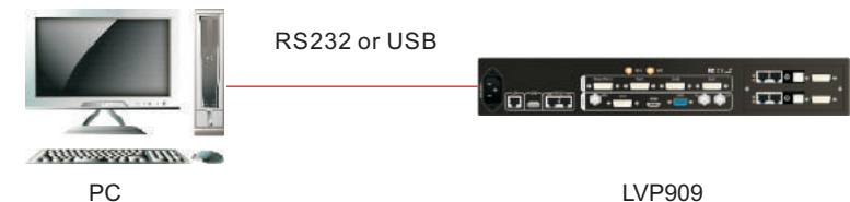
Pic 8-1b PC connection by USB / RS232
