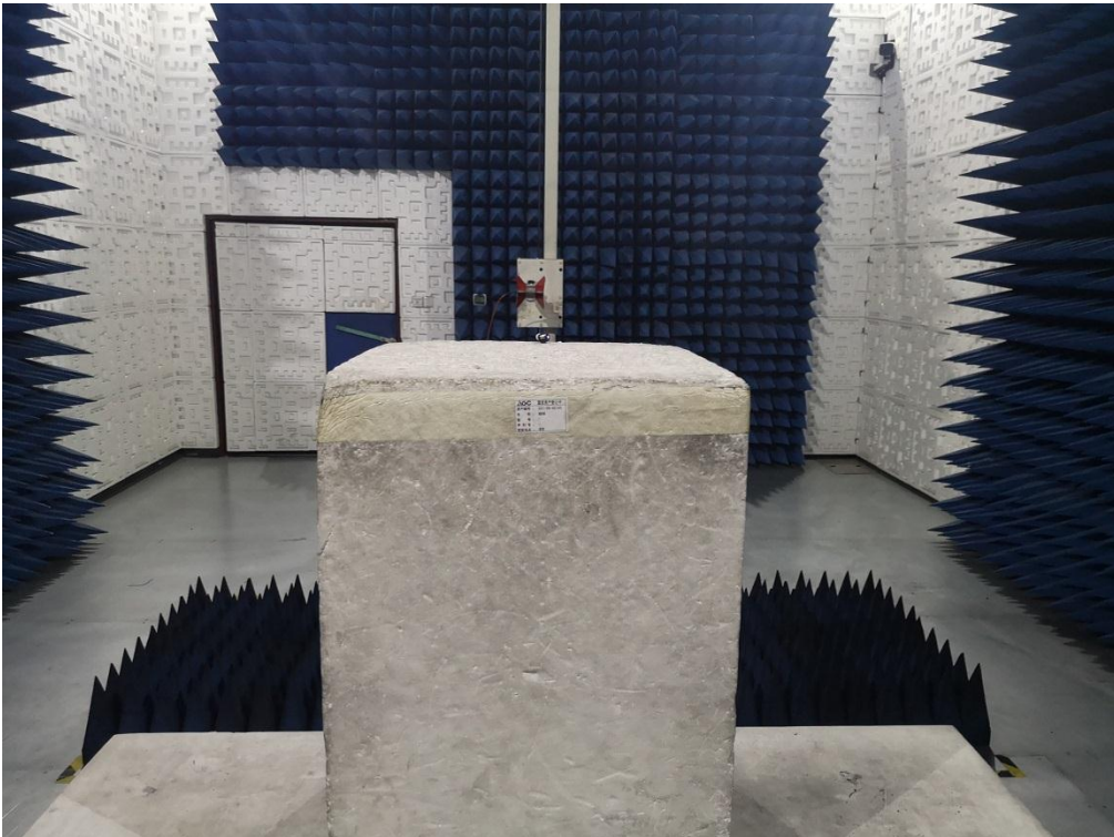
RADIATED EMISSION TEST SETUP ABOVE 1GHz
