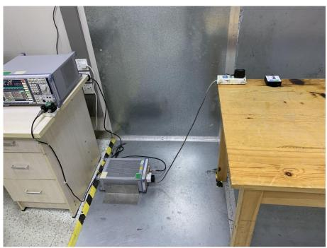
Radiated Spurious Emissions From 30MHz-1000MHz
