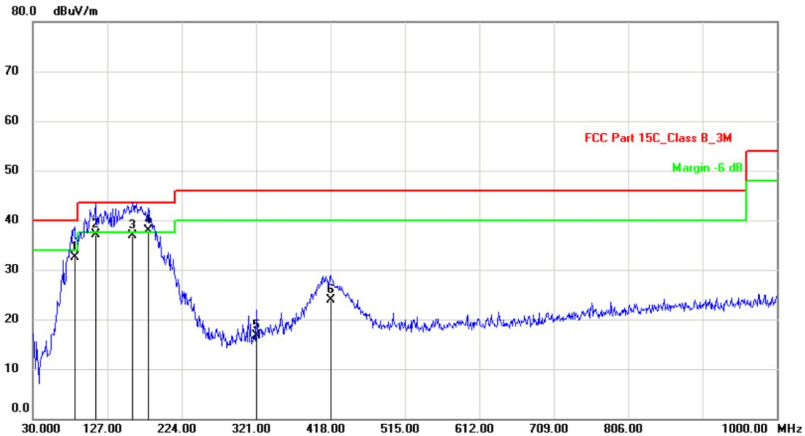
Site Polarization: *Horizontal* Temperature: 26
