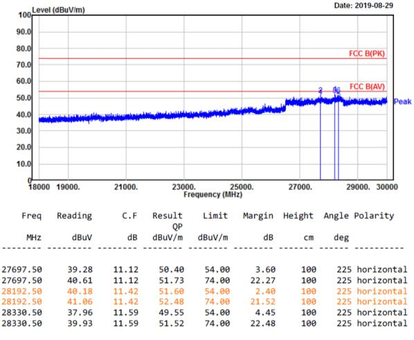
Remarks: C.F (Correction Factor) = Antenna factor + Cable loss - Preamp gain Note : Only the worst case plots for Radiated Spurious Emissions.
