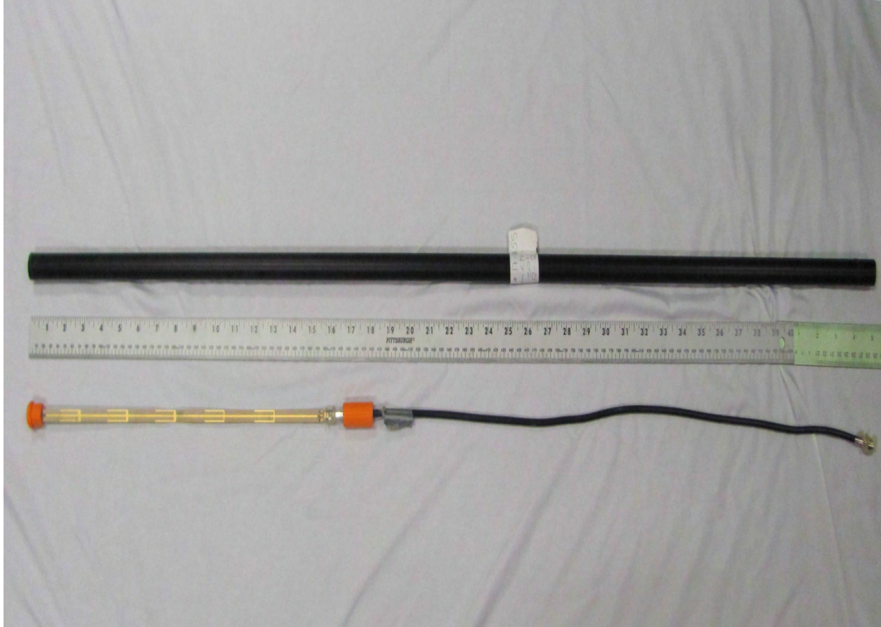
Figure 10. 2400 MHz Antenna outside of plastic cover
