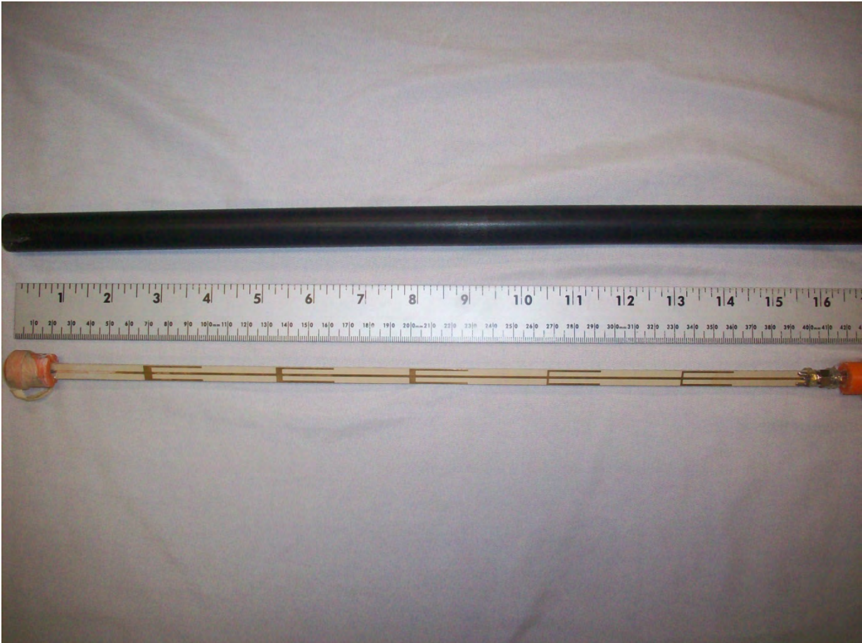
Figure 11. 2400 MHz Antenna Element
