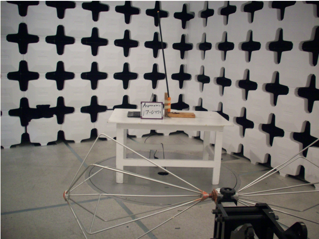
Figure 4. Spurious Radiated Emissions, 30-200 MHz
