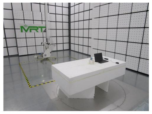
Test Mode: Mode 1~5 Description: Radiated Emission Test Setup for above 1GHz
