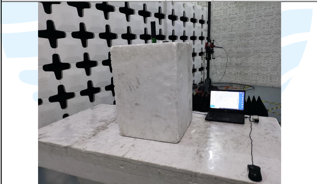
Radiated emission Test Setup (Above 1 GHz) For BLE
