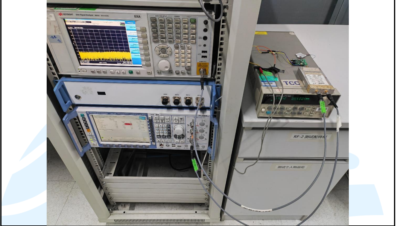
RF Conducted Test Setup For BR/EDR
