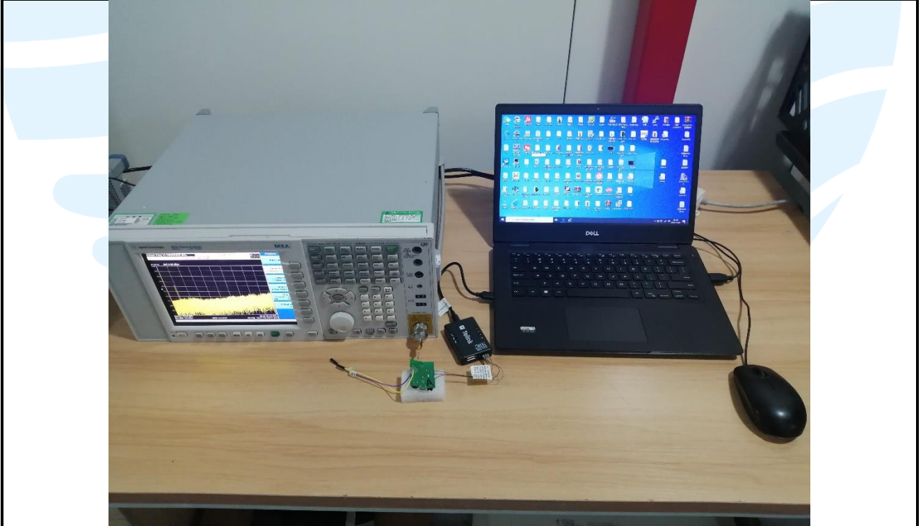
RF Conducted Test Setup For BLE
