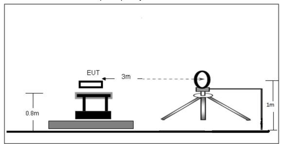
(B) Radiated Emission Test-Up Frequency 30MHz~1GHz
