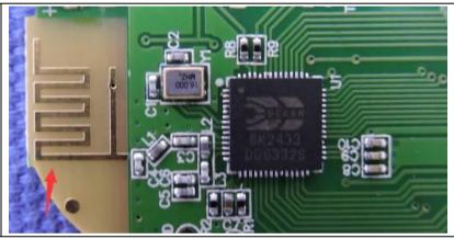
The antenna is integrated on the main PCB and no consideration of replacement. The best case gain of the antenna is 0dBi.
