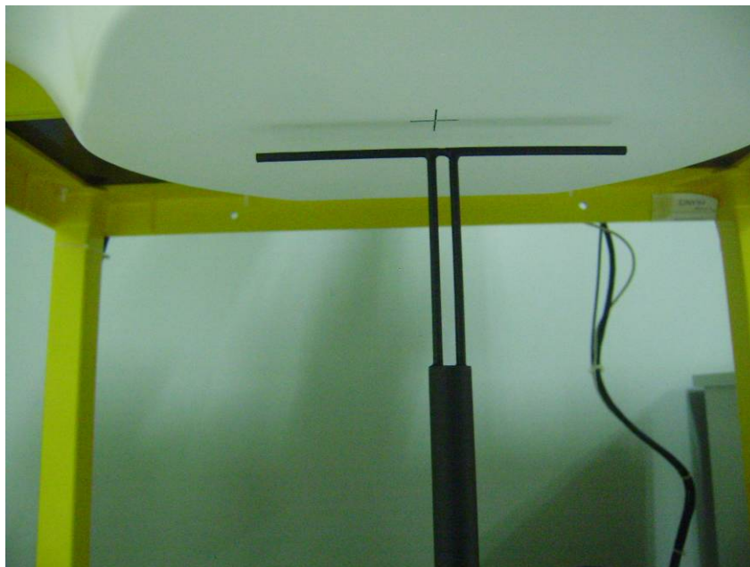
Fig 6.2 Setup Photo of Dipole Antenna
