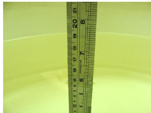
Fig 7.2 Photo of Liquid Height for Body SAR
