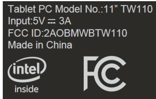
Specifications: Text is Black in color and justified. Labels are printed in indelible ink on permanent adhesive silk-screened onto the EUT or shall be affixed at a conspicuous location on the EUT.
