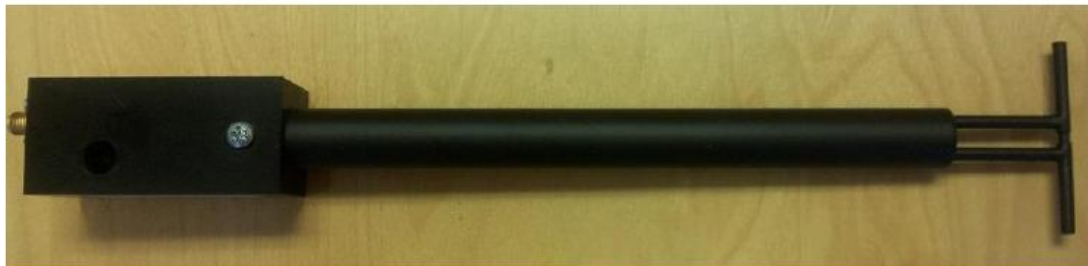
Figure 1 – MVG COMOSAR Validation Dipole
