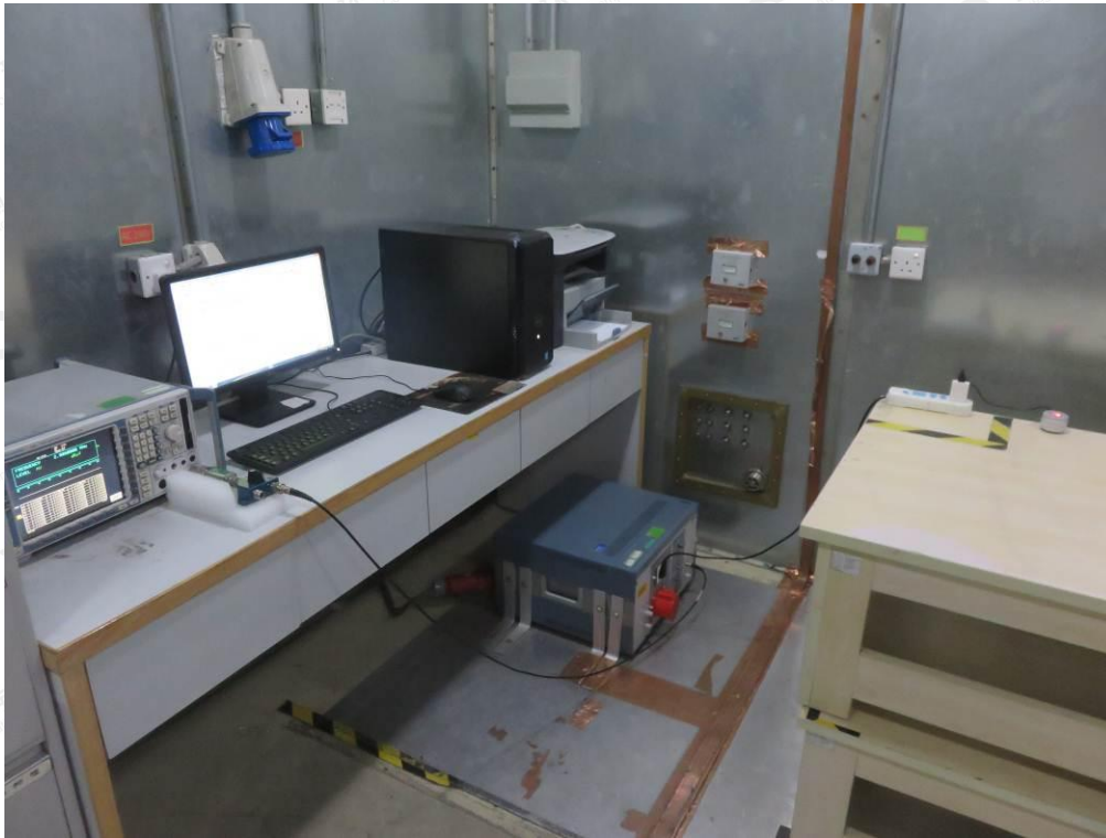
FCC RADIATED EMISSION TEST SETUP
