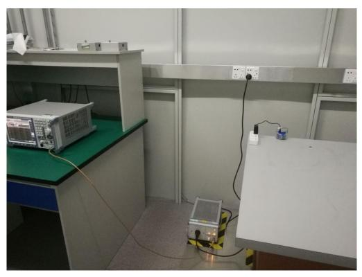
FCC RADIATED EMISSION TEST SETUP
