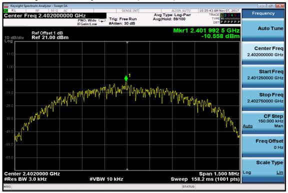
**Power Spectral Density Test Plot (CH-Mid)**
