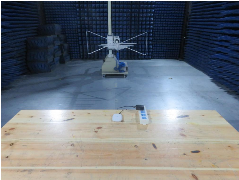
Photo of Radiation Emission Test
