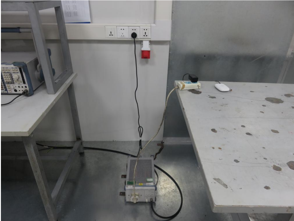
Photo of Conducted Emission Measurement
