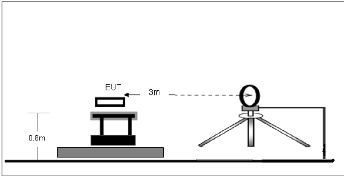
Radiated Emission Test-Up Frequency 30MHz~1GHz
