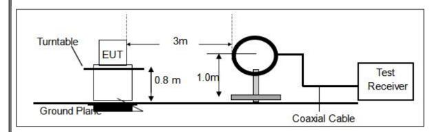
b) For Radiated Emission 30~1000MHz
