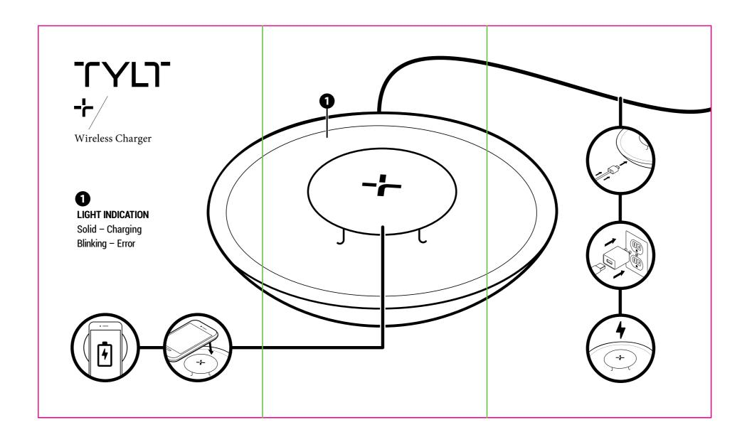
This is a wireless charger that will charge any device that supports the Qi standard, Please read the user manual before using and keep itfor future reference.
