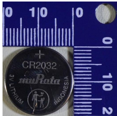
Figure 8 - Industrial Edge Machine - RTC Backup Battery
