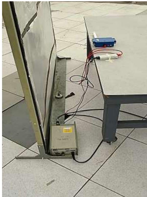
PoE Test Setup; Side View
