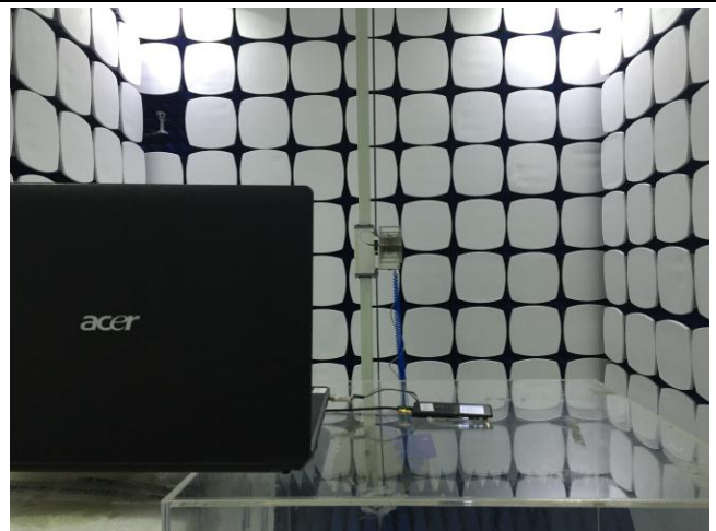
Radiated Spurious Emissions Test Setup Above 1GHz
