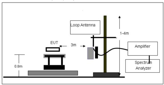
(B) Radiated Emission Test-Up Frequency 30MHz~1GHz
