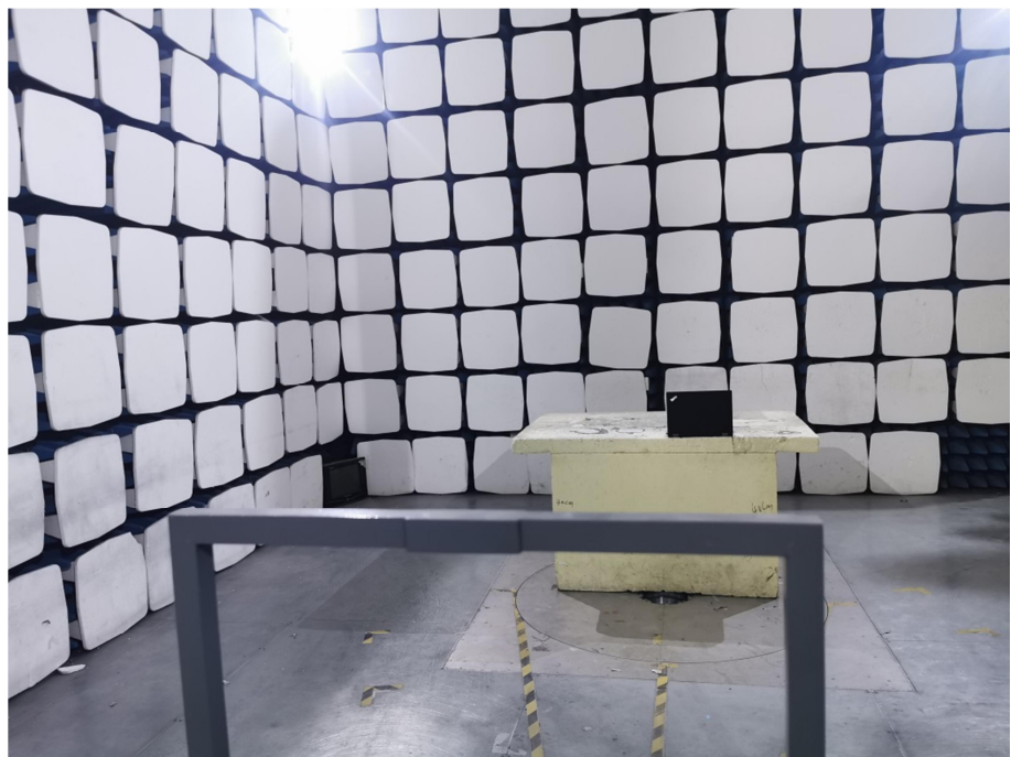
Radiation Emission Test Setup (Below 30MHz)
