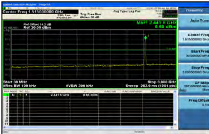
802.11g: Spurious Emission Test Data CH-Mid
