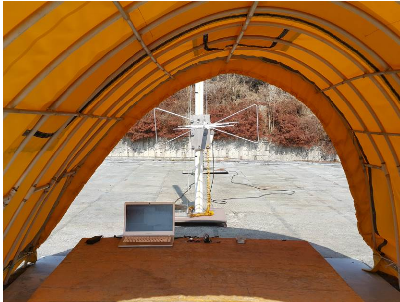
Photograph 1 : Setup for radiated Emissions (above 30 MHz)
