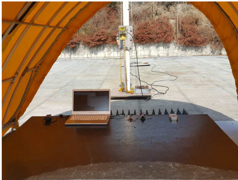
Photograph 2 : Setup for radiated Emissions (above 1 GHz)
