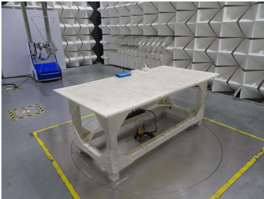
Radiated spurious emission Test Setup-2(30MHz-1GHz)
