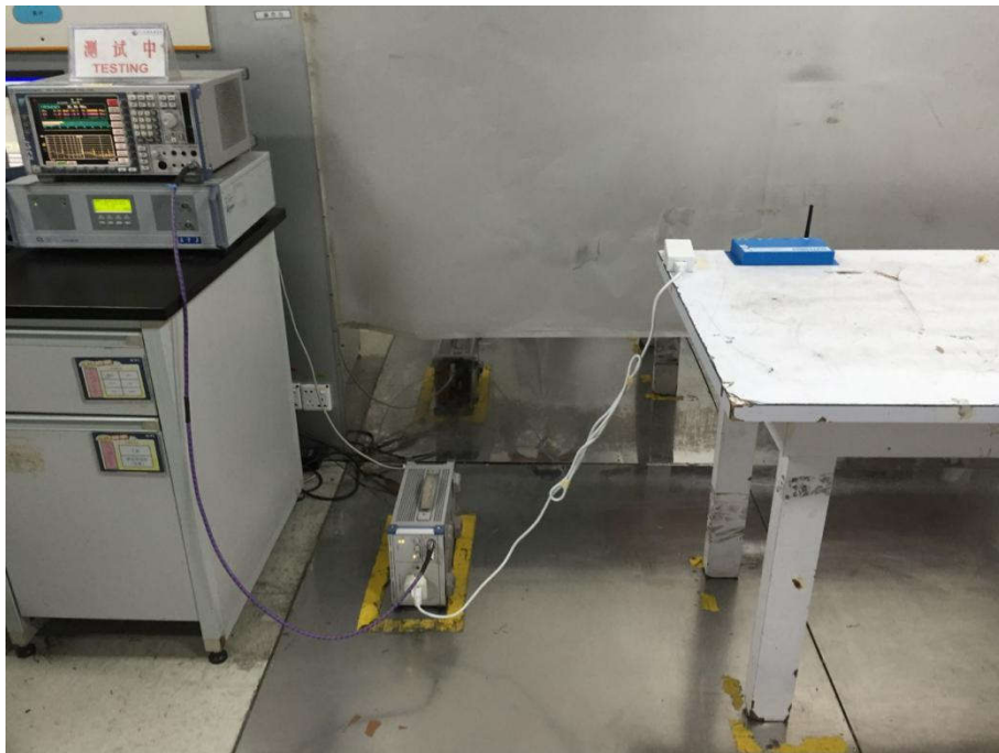
Conducted Emissions Test Setup
