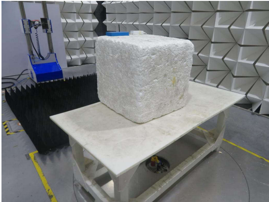
Radiated spurious emission Test Setup-3(Above 1GHz)
