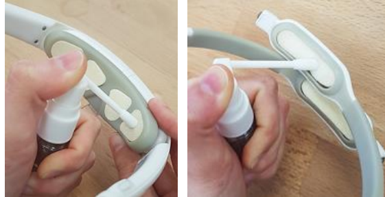
Figure 22: Wetting the Electrode Pads
