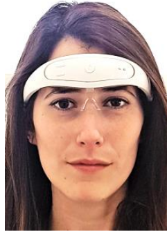
Figure 26: Proper Placement of Front Part of the Device
