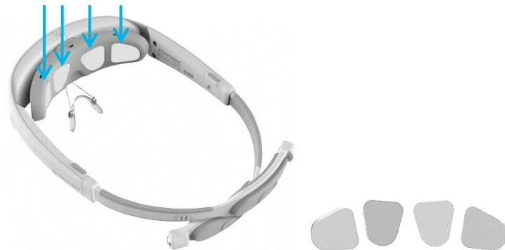
Figure 8: Front Electrode Pads
