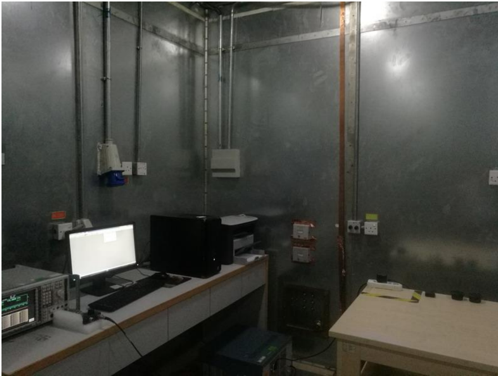
FCC RADIATED EMISSION TEST SETUP
