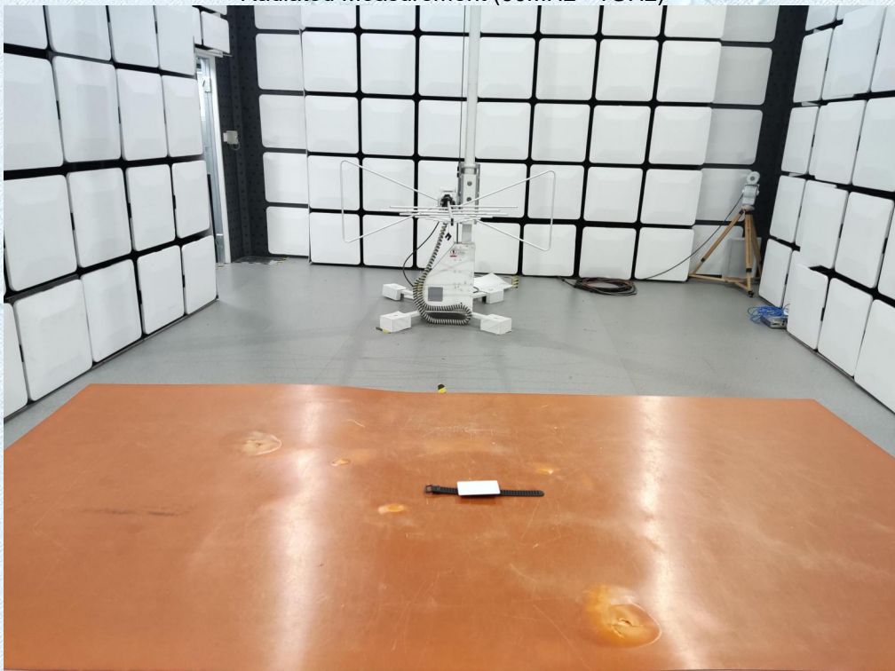
Radiated Measurement (30MHz~ 1GHz)
