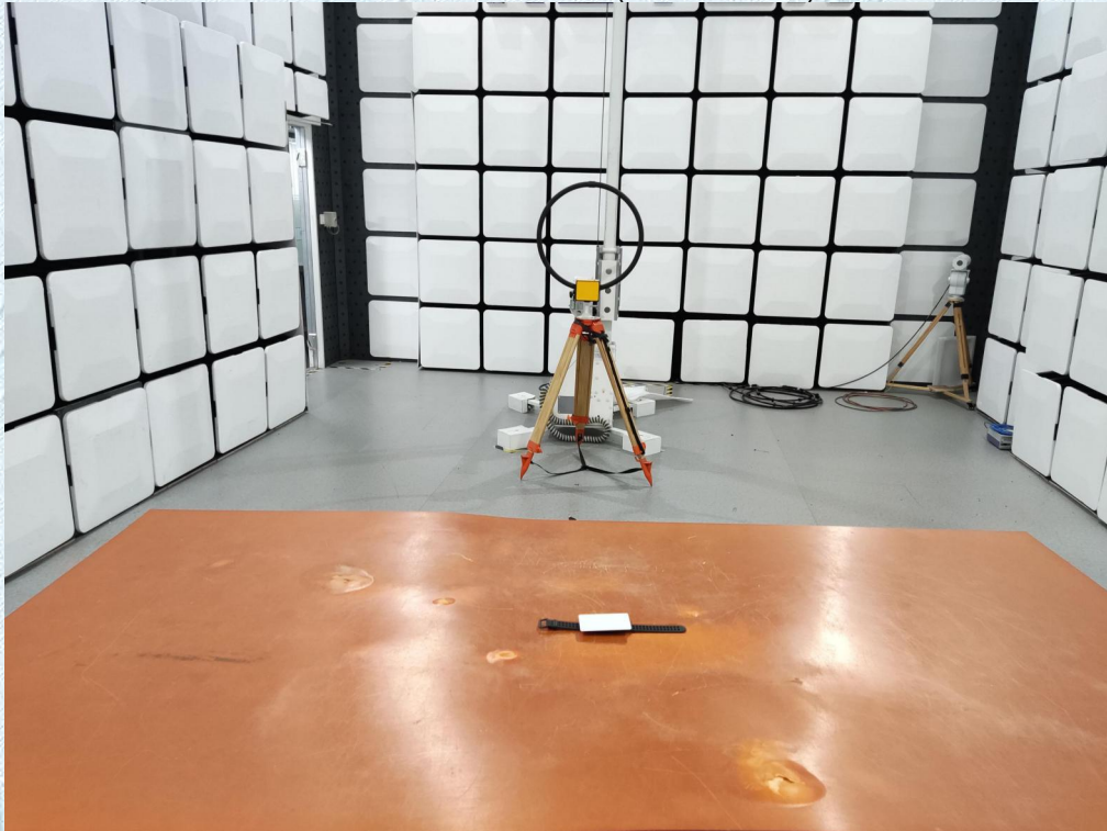
Radiated Measurement (30MHz~ 1GHz)
