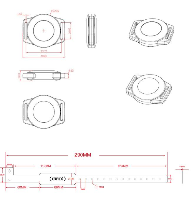
Notes: 1.All units is mm. 2.No RFID by default, RFID can be customized on the wristband or Beacon.
