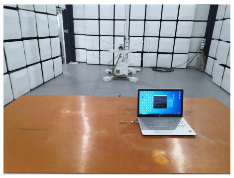
Radiated Measurement (Above 1GHz)
