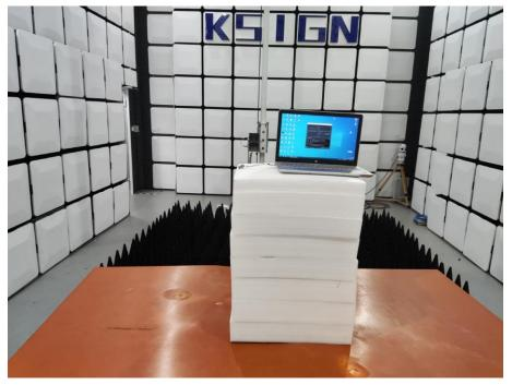
CONDUCTED EMISSION TEST SETUP
