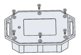
Step1: Remove the screws on the bottom of the device
