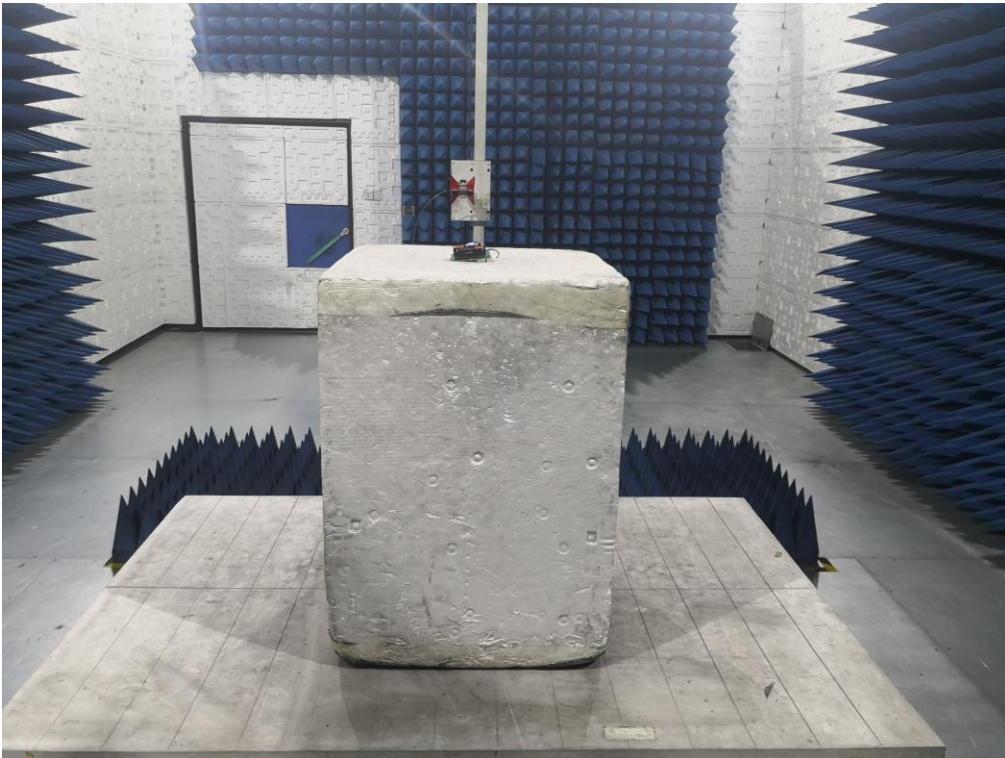
RADIATED EMISSION TEST SETUP ABOVE 1GHZ
