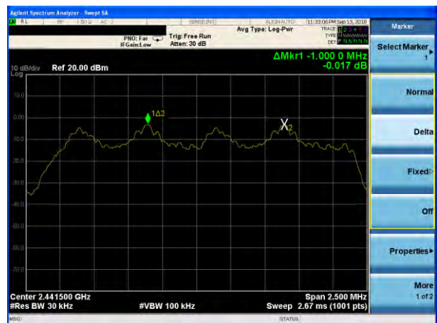
(2Mbps) Channel Separation plot on channel 39-40
