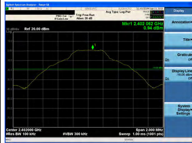
GFSK on channel 00
