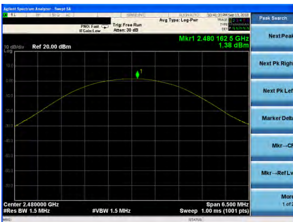
Peak output Power plot on channel 78 (3Mbps)
