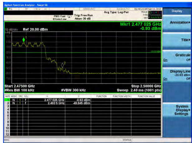
8-DPSK: Band Edge-High Channel (Hopping Mode)
