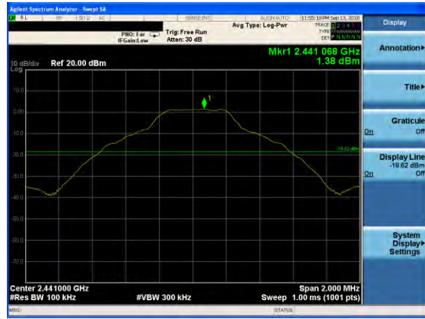
GFSK on channel 39
