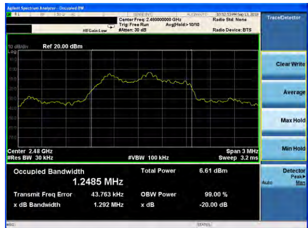
20dB Bandwidth plot on channel 78 (2Mbps)
