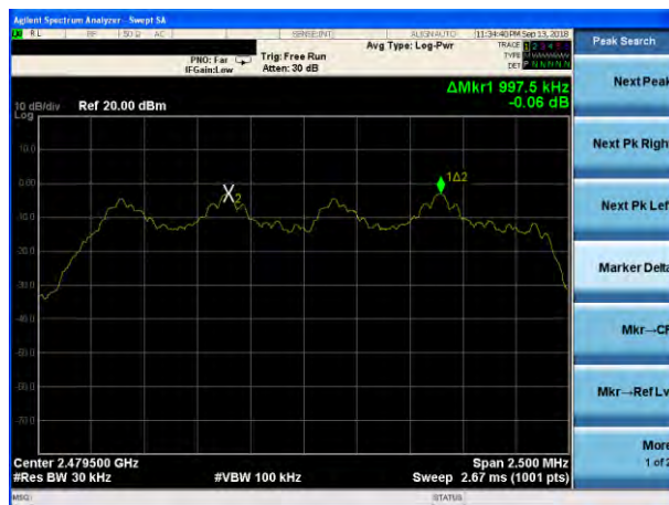
(2Mbps) Channel Separation plot on channel 77-78
