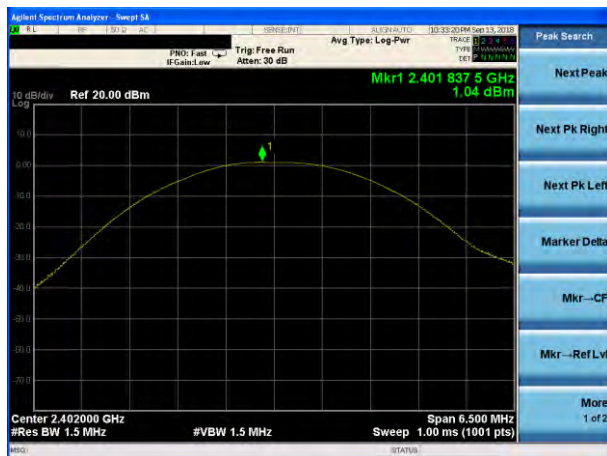
Peak output Power plot on channel 39 (2Mbps)
