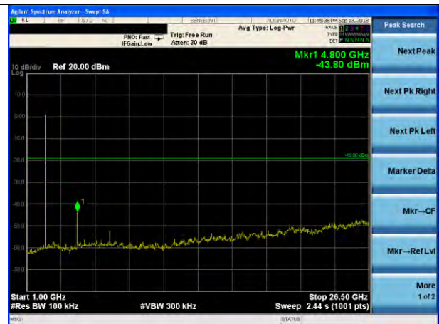
GFSK on channel 00
