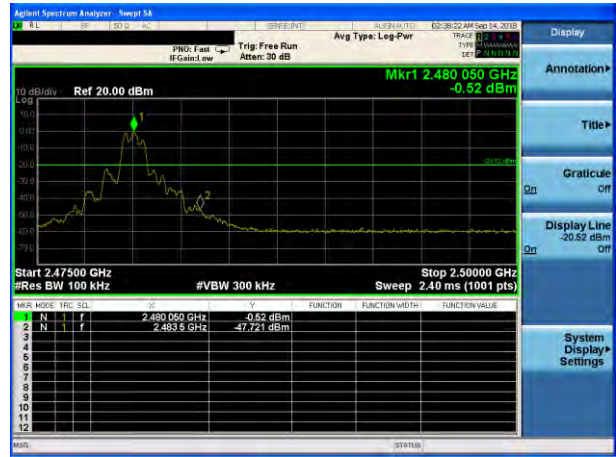
8-DPSK: Band Edge-High Channel
