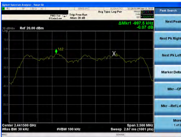
(3Mbps) Channel Separation plot on channel 77-78
