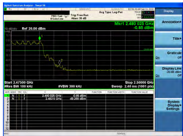
\pi /4-DQPSK: Band Edge-High Channel (Hopping Mode)
