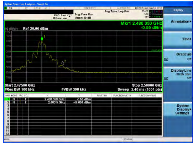
8-DPSK: Band Edge-High Channel
