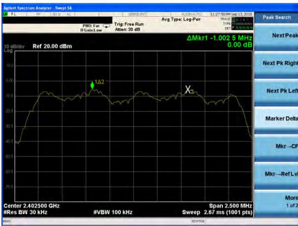
(3Mbps) Channel Separation plot on channel 39-40
