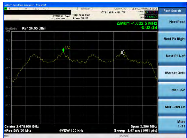
(2Mbps) Channel Separation plot on channel 77-78
