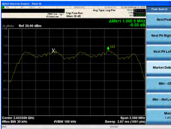
(3Mbps) Channel Separation plot on channel 39-40
