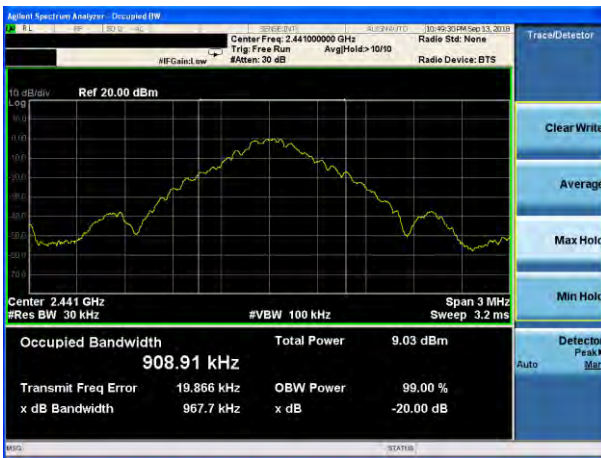
20dB Bandwidth plot on channel 39 (1Mbps)
