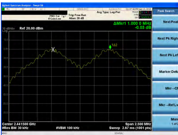
(1Mbps) Channel Separation plot on channel 39-40
