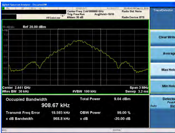
20dB Bandwidth plot on channel 78 (1Mbps)
