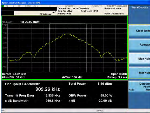
20dB Bandwidth plot on channel 39 (1Mbps)
