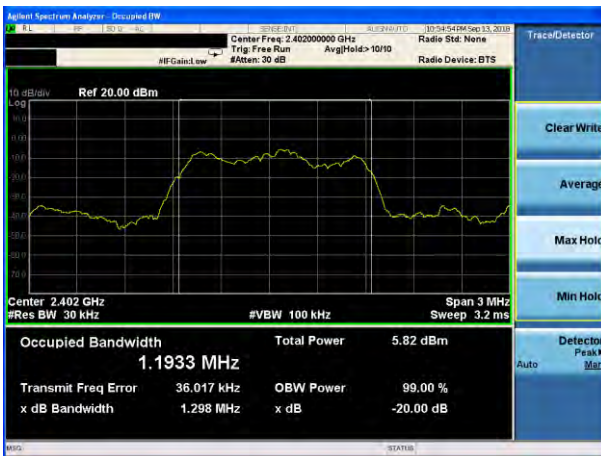
20dB Bandwidth plot on channel 00 (3Mbps)
