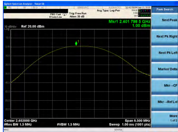
Peak output Power plot on channel 39 (2Mbps)
