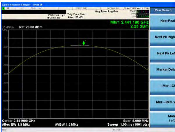
Peak output Power plot on channel 39 (1Mbps)
