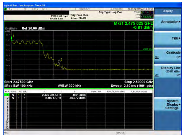
\pi /4-DQPSK: Band Edge-High Channel (Hopping Mode)
