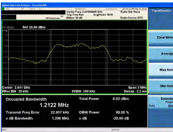
20dB Bandwidth plot on channel 39 (3Mbps)
