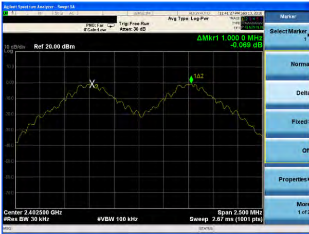
(1Mbps) Channel Separation plot on channel 39-40
