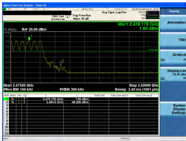
GFSK: Band Edge-High Channel (Hopping Mode)
