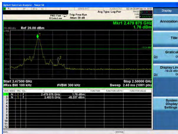
GFSK: Band Edge-High Channel (Hopping Mode)
