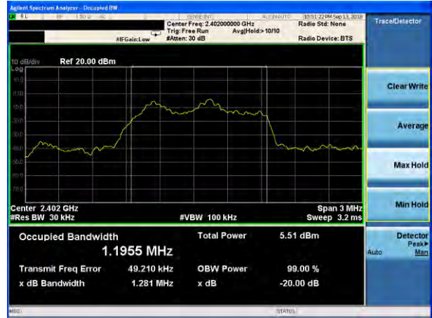
20dB Bandwidth plot on channel 39 (2Mbps)
