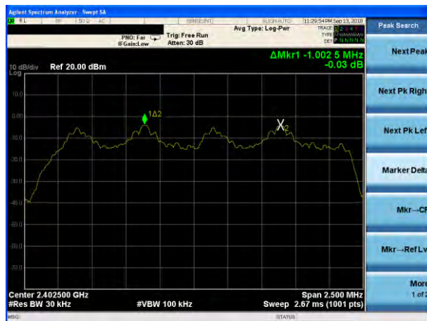
(2Mbps) Channel Separation plot on channel 39-40
