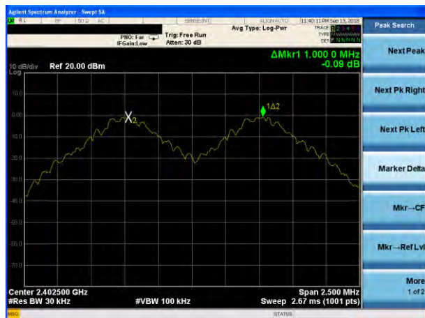
(1Mbps) Channel Separation plot on channel 39-40
