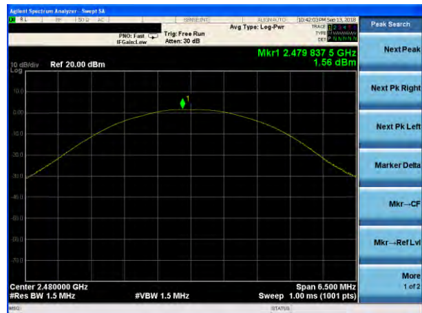
Peak output Power plot on channel 78 (2Mbps)
