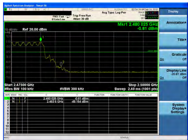
8-DPSK: Band Edge-High Channel (Hopping Mode)
