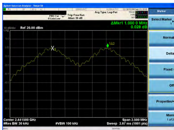
(1Mbps) Channel Separation plot on channel 39-40
