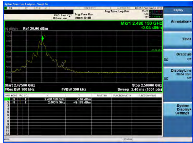
\pi /4-DQPSK: Band Edge-High Channel (Hopping Mode)
