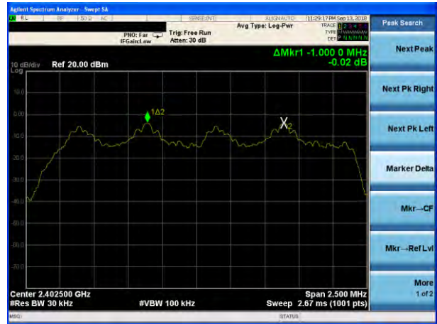
(2Mbps) Channel Separation plot on channel 39-40
