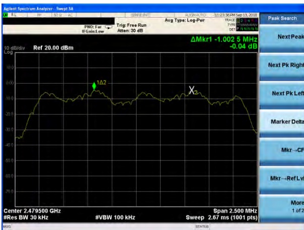
(3Mbps) Channel Separation plot on channel 77-78
