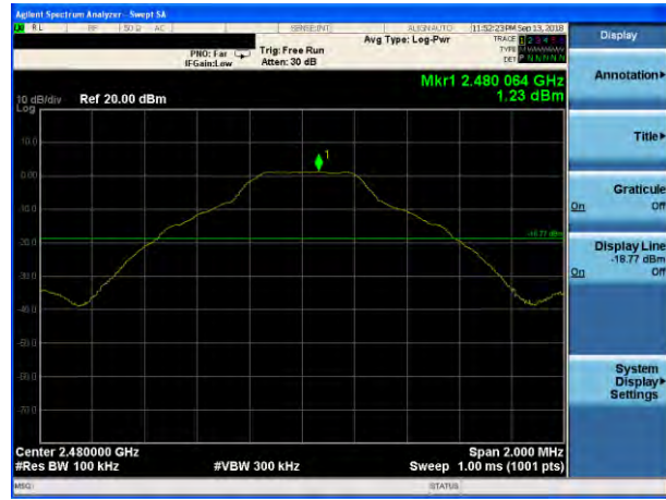
GFSK on channel 78
