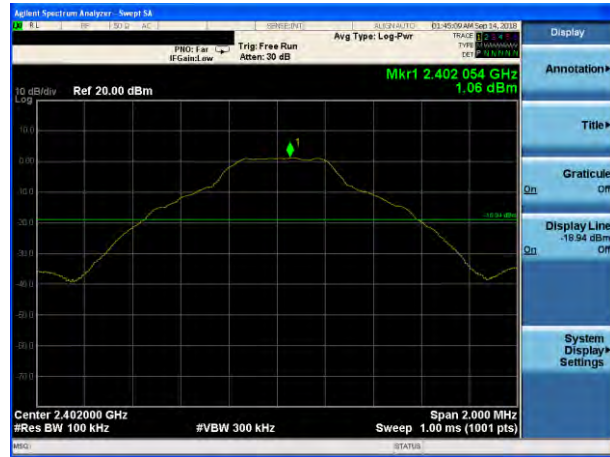
GFSK on channel 00
