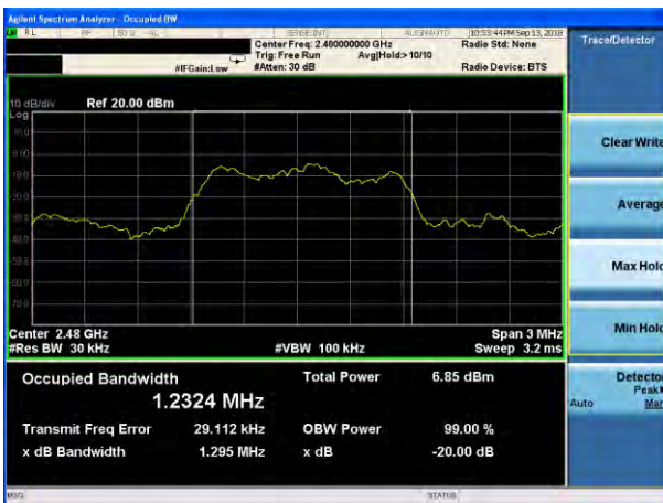
20dB Bandwidth plot on channel 78 (3Mbps)
