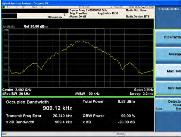
20dB Bandwidth plot on channel 39 (1Mbps)
