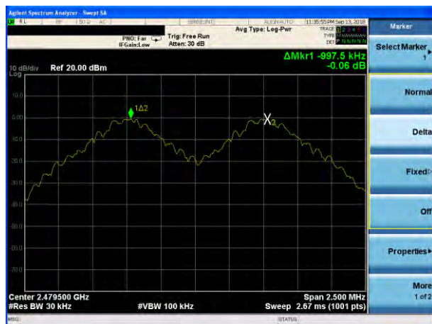
(1Mbps) Channel Separation plot on channel 77-78
