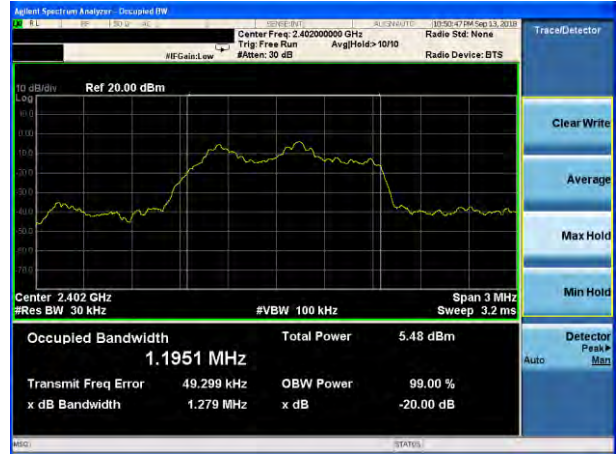
20dB Bandwidth plot on channel 39 (2Mbps)
