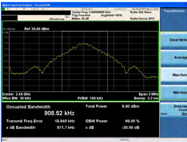
20dB Bandwidth plot on channel 78 (1Mbps)
