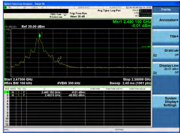
\pi /4-DQPSK: Band Edge-High Channel (Hopping Mode)
