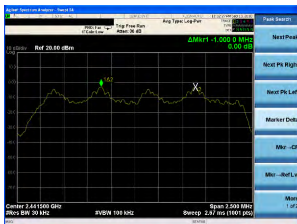
(2Mbps) Channel Separation plot on channel 39-40
