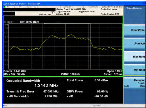
20dB Bandwidth plot on channel 39 (2Mbps)
