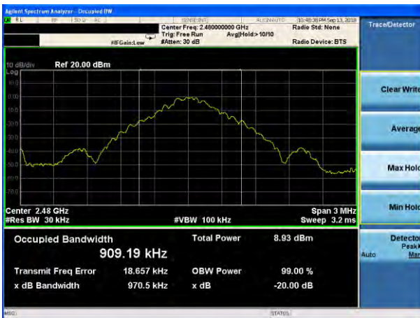
20dB Bandwidth plot on channel 78 (1Mbps)
